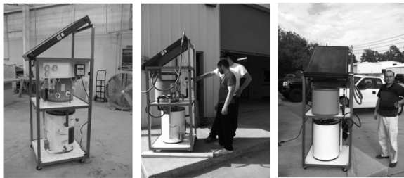
Figure 3. Solar thermal water heating system
