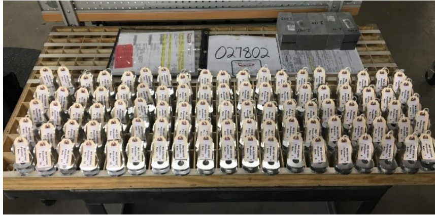
Figure 3. Special tray used to record the measurement and position on fixture
