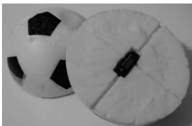
Figure 2. Foam soccer ball with the wireless Bluetooth® sensor. The sensor was capable of acquiring altitude and acceleration about 3-axes.
